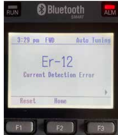
Typical auto-tuning fault
